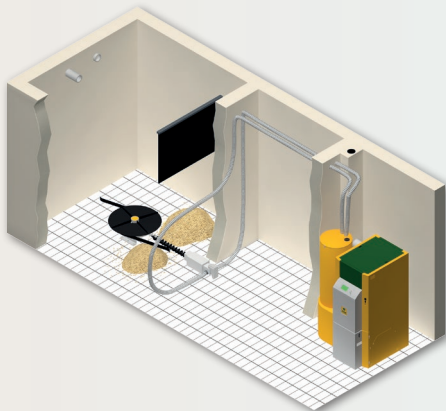
Pellet Stirrer Plus with suction conveyor
